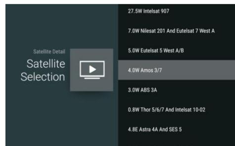
Turn Satellite Status on, Setting satellite parameters or Click Satellite Selection to select other satellites. After adding, you need return to satellite Re-Scan for Satellite scan.
