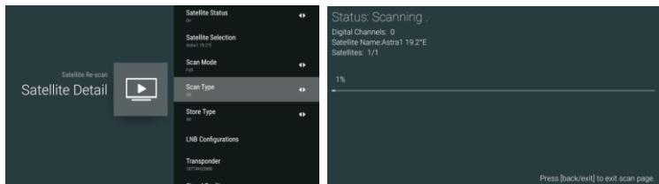
Press OK to enter the Satellite parameter Settings, which include LNB POWER, LNB Frequency, DiSEqC Set, 22K and other parameters.
